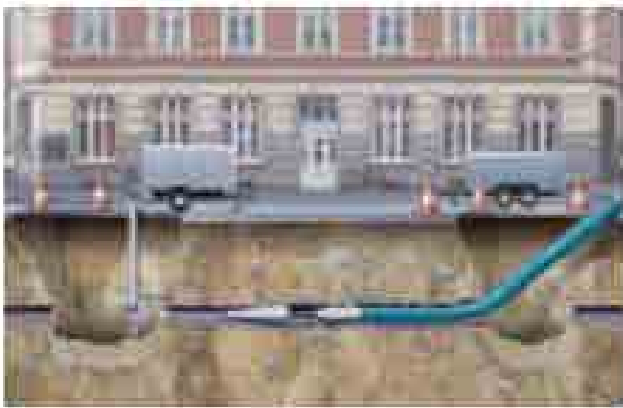
Afb. 2-10 Dynamische berstlining (Pipe Cracking)
